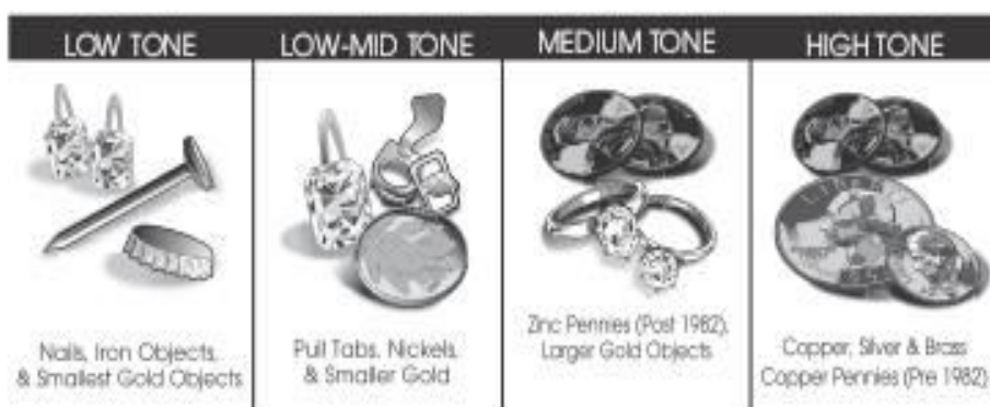
Audio Target Identification (ATI) classifies metals into four categories.
